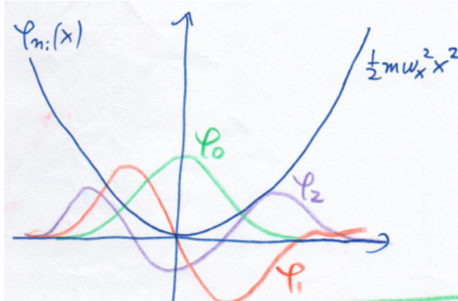
left: Sketch of 1D harmonic oscillator potential and the first few eigenstates
