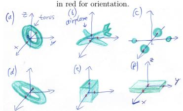
top: (a) Regular circular torus. (b) Airplane, with the usual pieces and symmetries. (c) 4 Spheres, 2 large, 2 small, all the same distance from the origin. (d) Ellipsoidal torus, with smaller radius along x-axis. (e) Symmetric cube. (f) Cuboid, with withs along axes  $w_z < w_x < w_y$ .
