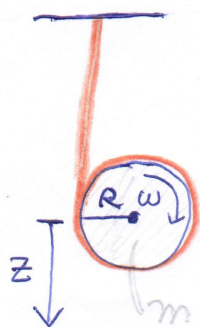
Figure 1: Sketch of yoyo. A string (brown) is held with your finger and wound around a cylinder (grey) of mass m with radius R . The yoyo can move down by unwinding the string while rotating, and up by winding up the string through rotation.
