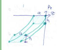
**left:** We see from Eq. (4.29) that the momentum difference between two phase-space points never changes compared to the initial value. For two trajectories with equal initial momentum, also the position difference never changes. Overall, a phase space volume such as the green one thus changes from rectangular into parallelogram, but the base-width a and height h remain constant, and hence the volume V = ah does not change.
